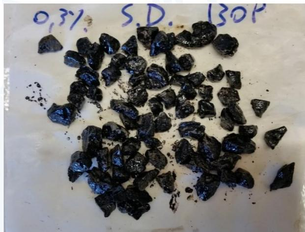
Figure 4a. Results Boiling Water Stripping Test basalt aggregates: left bitumen without additive, right bitumen with the addition of 0.3% StarDope® 130 P.
