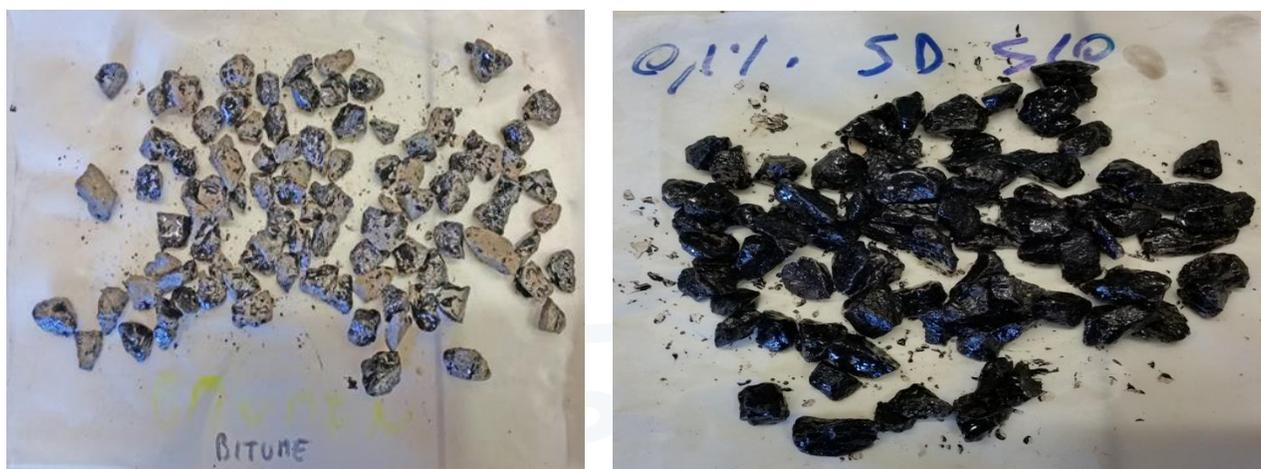
Figure 6a. Results Boiling Water Stripping Test basalt aggregates: left bitumen without additive, on the right bitumen with the addition of 0.1% of StarDope® 510.
