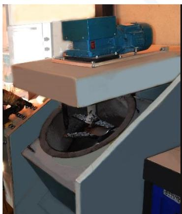
The mixtures were packaged in the laboratory by means of a thermostatic mixer for asphalt (Infratest), using a percentage of 5% by weight binder referred to the inerts. The Asphalt mix were made by dosing the additives in variable percentages between 0.4 and 0.6% on the weight of the binder.
