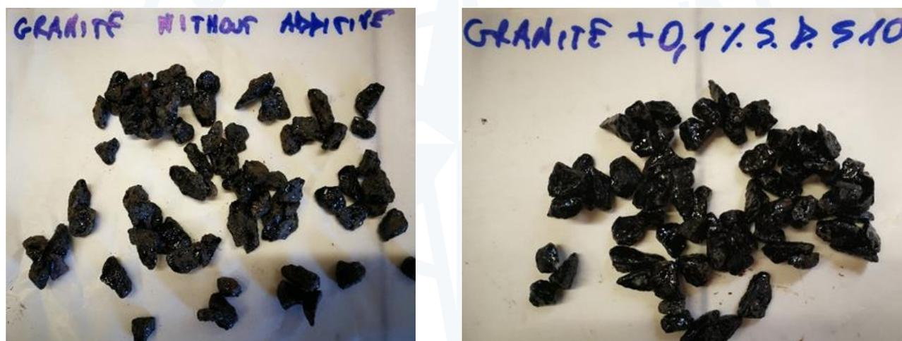
Figure 6b. Results Boiling Water Stripping Test inert granites: left bitumen without additive, on the right bitumen with the addition of 0.1% of StarDope® 510.
