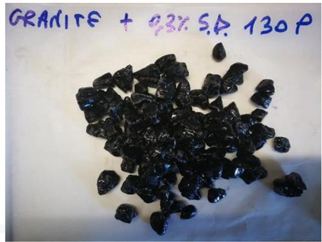
Figure 4f. Results Rolling Bottle Test inert granites: on the left bitumen without additive, on the right bitumen with the addition of 0.3% of StarDope® 130 P.
