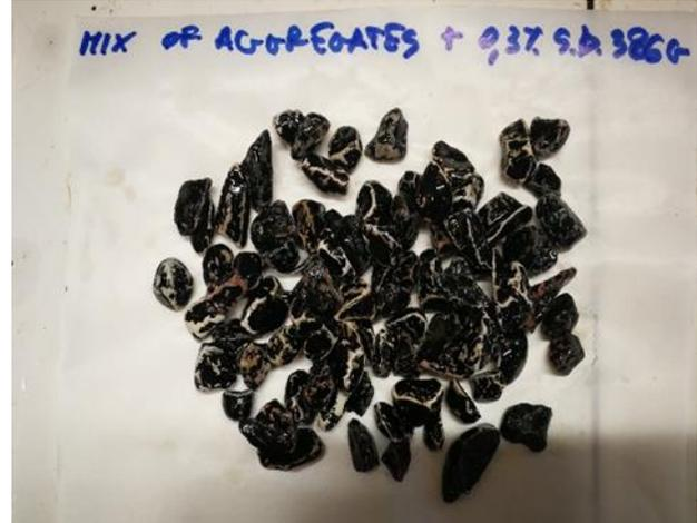
Figure 5h. Results Rolling Bottle Test aggregate mix: left bitumen without additive, on the right bitumen with the addition of 0.3% of StarDope® 386 G.
