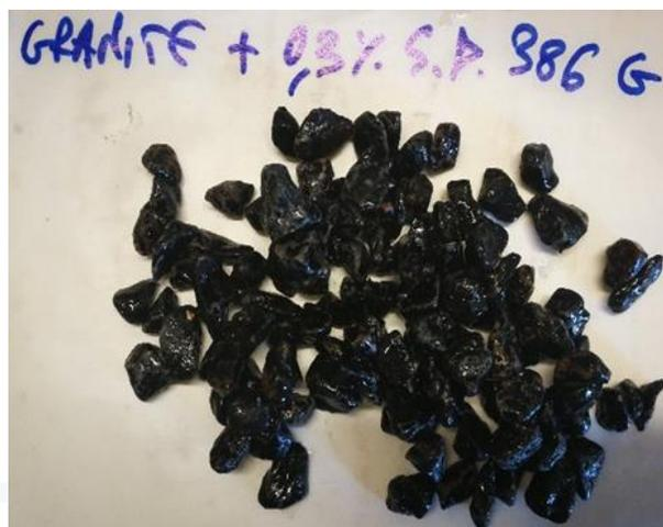
Figure 5f. Results Rolling Bottle Test inert granites: left bitumen without additive, on the right bitumen with the addition of 0.3% of StarDope® 386 G.
