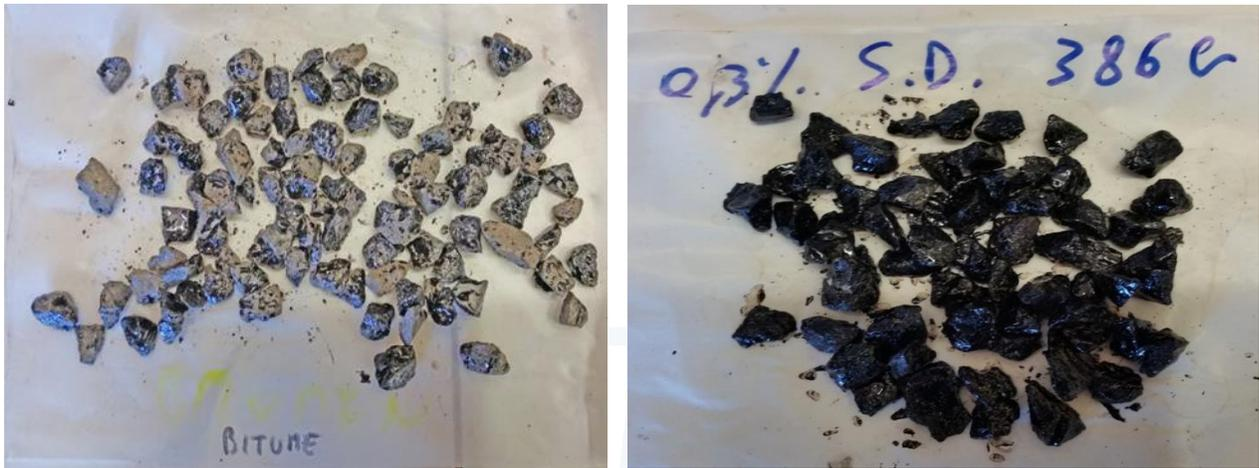
Figure 5a. Results Boiling water stripping Test basalt aggregates: left bitumen without additive, on the right bitumen with the addition of 0.3% of StarDope® 386 G.
