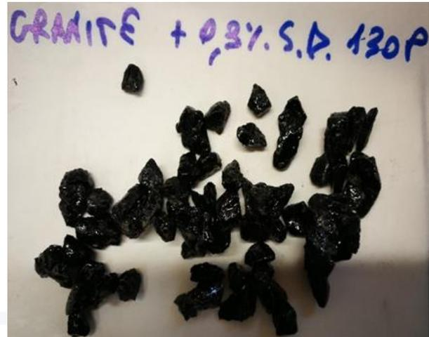
Figure 4b. Results Boiling Water Stripping Test inert granites: left bitumen without additive, right bitumen with the addition of 0.3% of StarDope® 130 P.
