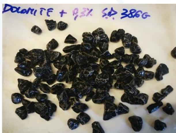
Figure 5g. Results Rolling Bottle Test inert dolomitics: left bitumen without additive, on the right bitumen with the addition of 0.3% of StarDope® 386 G.
