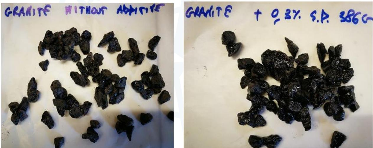
Figure 5b. Results Boiling water stripping Test inert granites: left bitumen without additive, on the right bitumen with the addition of 0.3% of StarDope® 386 G.
