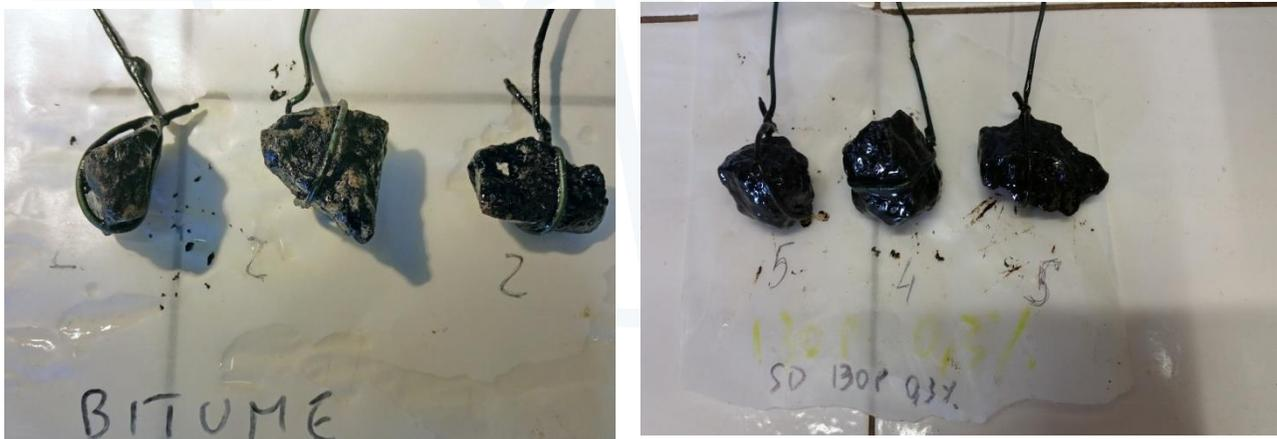
Figure 4i. Results Granitic inert tests: left bitumen without additive, on the right bitumen with the addition of 0.3% of StarDope® 130 P.
