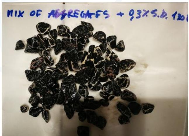
Figure 4h. Results Rolling Bottle Test aggregate mix: left bitumen without additive, right bitumen with the addition of 0.3% StarDope® 130 P.
