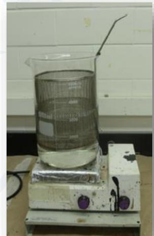
The second technique involves placing test samples inside glass containers filled with water at room temperature. These containers are rotated and shaken for a variable period of time (up to 24 hours) and inspected every 6 hours giving a visual assessment of the degree of bitumen coverage, as a percentage of the aggregates.
