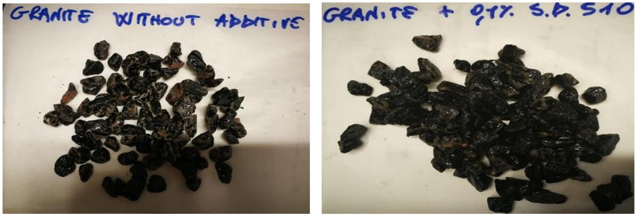
Figure 6f. Results Rolling Bottle Test inert granites: on the left bitumen without additive, on the right bitumen with the addition of 0.1% of StarDope® 510.
