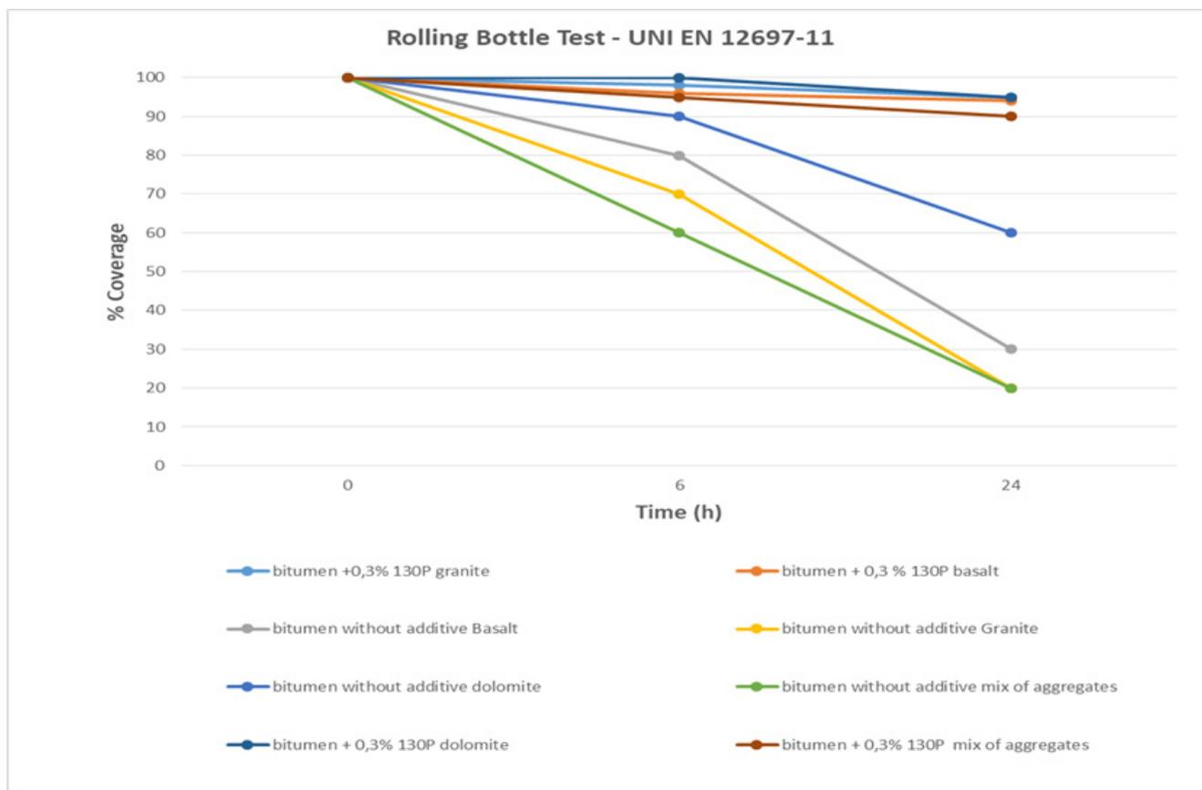
• Rolling Bottle Test Chart StarDope® 130 P vs Non-Additive at t = 6h.
