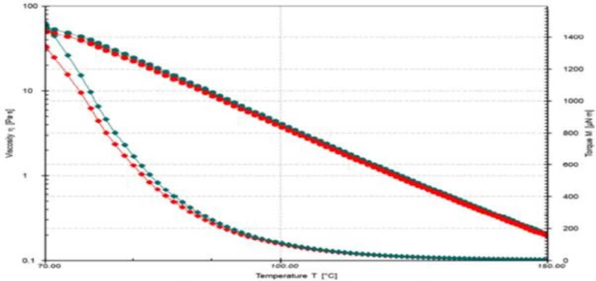
Graph 3. Overlap of curves of bitumen samples without additive and with 0.5% of Warm-Mix® L with shear rate = 0.5s<sup>-1</sup> in a range of T=70-150°C.
