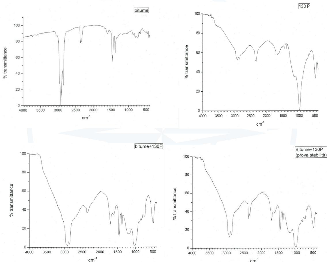
Figure 4l. Infrared spectrum acquired in transmittance by Fourier Transform Infrared Spectrometer in the frequency range between 4000 and 400 cm<sup>-1</sup>.
