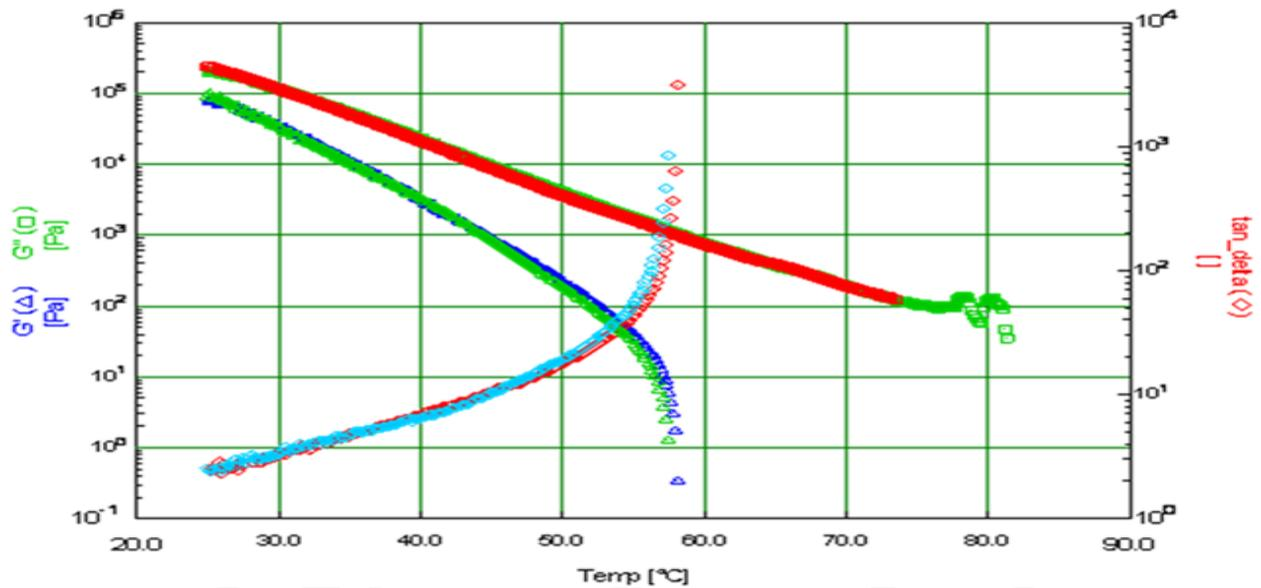
Graph 1. Storage module ( $G'$ ) and loss module ( $G''$ ) of a non-additive bitumen and of a bitumen additived with 0.5% of Warm-Mix® L. Department of Chemistry - UNIVERSITY OF CALABRIA - Arcavacata di Rende.
