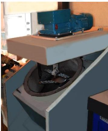
The mixtures were packaged in the laboratory by means of a thermostatic mixer for bituminous conglomerates (Infratest), using a total percentage of binder of 4.5% by weight referred to the inerts (old + new bitumen). 30% rap were made, dosing the additive to 0.2 and 0.3% respectively on the weight of the milled product.
