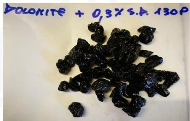
Figure 4c. Results Boiling Water Stripping Dolomites inert tests: left bitumen without additive, on the right bitumen with the addition of 0.3% of StarDope® 130 P.
