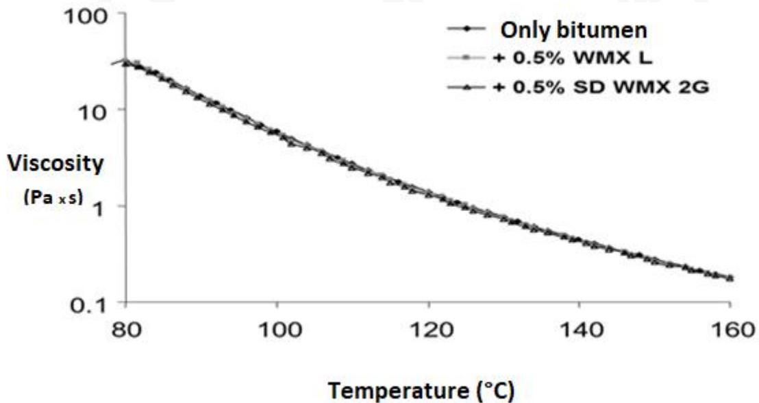
Graph 4. Trend of the viscosity as a function of the temperature of a sample of non-mixed bitumen, a sample of bitumen with 0.5% of Warm-Mix® L and a sample of bitumen added with 0.5% of StarDope® Warm-Mix 2G: as you can see, all the curves are superimposed, indicating that there is no change in the viscosity of the bitumen as these additives do not modify the physical properties of the bituminous binder.
