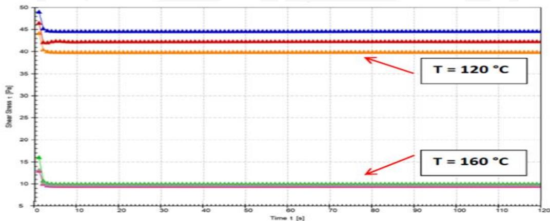
Graph 2. Overlap of "stress" curves of a sample of non-additive bitumen (blue curve), a sample of bitumen added with 0.5% of Warm-Mix® L (red curve) and a sample of bitumen admixed with 0.5% of StarDope® Warm-Mix 2G (orange curve) with deformation  $\gamma = 70\%$ , frequency  $\nu = 10$  Hz and temperature  $T=120^\circ\text{C}$  and  $T=160^\circ\text{C}$ .
