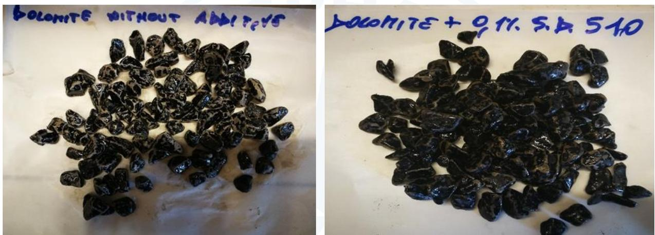
Figure 6g. Results Rolling Bottle Test inert dolomitic: left bitumen without additive, on the right bitumen with the addition of 0.1% of StarDope® 510.
