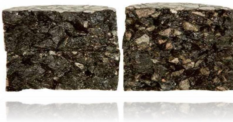
*Fig. 3. Section of a sample: on the left, a section of the sample made with adhesion promoter, on the right a section of the sample made without adhesion promoter.*
