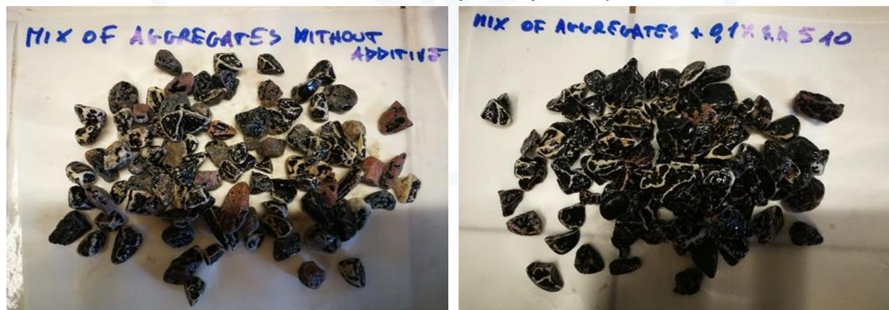
Figure 6h. Results Rolling Bottle Test inert mix: left bitumen without additive, on the right bitumen with the addition of 0.1% of StarDope® 510.
