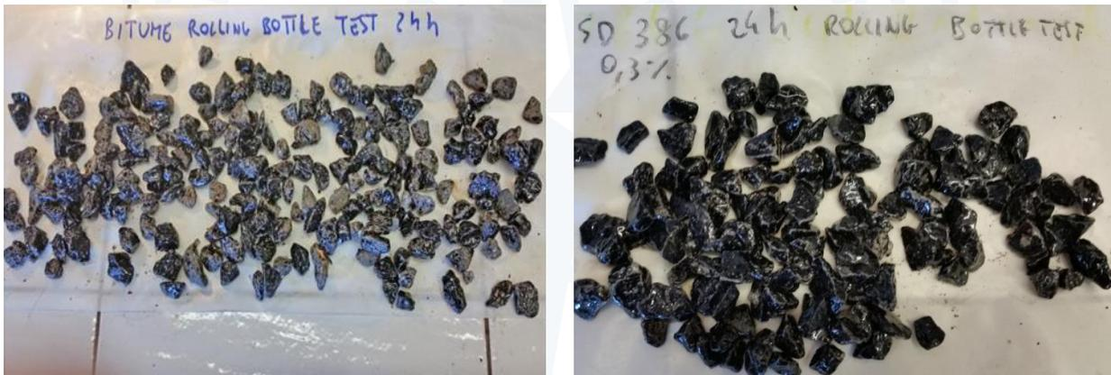
Figure 5e. Results Rolling Bottle Test inert basalt: on the left bitumen without additive, on the right bitumen with the addition of 0.3% of StarDope® 386 G.
