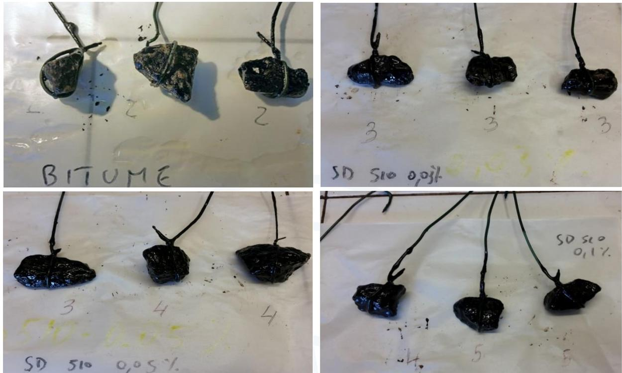
Figure 6i. Results Granitic inert tests: top left bitumen without additive, top right bitumen with the addition of 0.03% of StarDope® 510, lower left bitumen with the addition of 0.05% of StarDope® 510, in the lower right bitumen with the addition of 0.1% of StarDope® 510.
