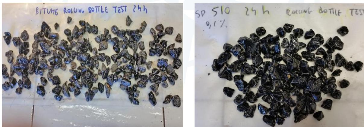
Figure 6e. Results Rolling Bottle Test inert basalt: on the left bitumen without additive, on the right bitumen with the addition of 0.1% of StarDope® 510.
