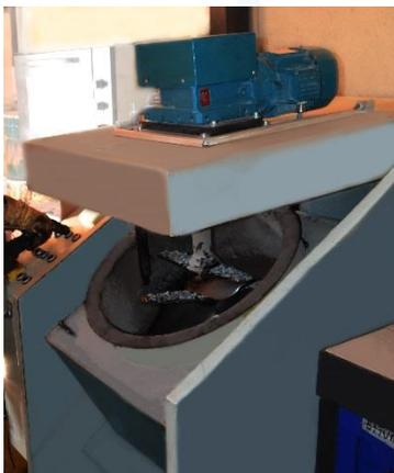
The mixtures were packaged in the laboratory by means of a thermostatic mixer for bituminous mixtures (Infratest), using a total percentage of 5% by weight binder referred to inerts (old + new bitumen). 40% and 50% milled bituminous conglomerates were made, dosing the additive ACF WARM-MIX® 40 to 0.37% and 0.41% respectively on the weight of the milled material.
